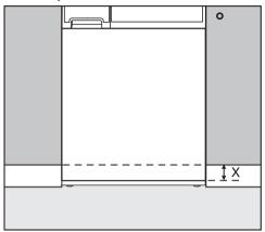
The measure **X** equals the space from the bottom of the washer door to the bottom of the adjacent cabinet.
